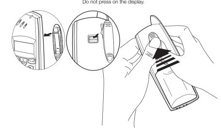
Attach the battery to the phone as shown in the figure below. Make sure that the battery wires are put through the notches as shown.
